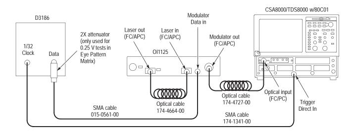
Figure 14: Setup for the RMS Jitter test
