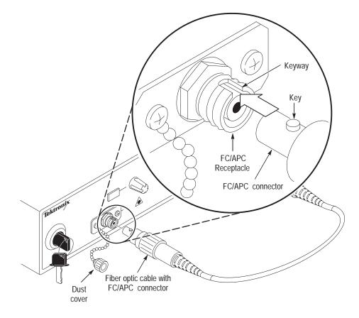
Figure 4: Connecting a fiber optic cable
