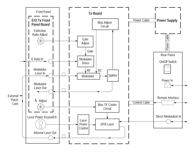
Figure 11: Transmitter interconnect diagram
