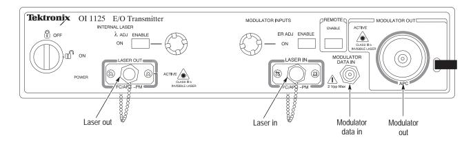
Figure 5: OI1125 front-panel connectors
