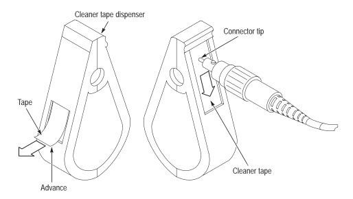
Figure 20: Cleaning an optical connector
