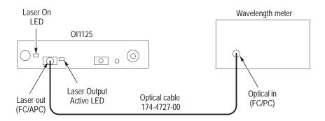
Figure 13: Setup for the output wavelength test
