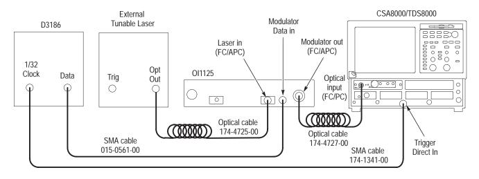
Figure 18: Setup for the eye pattern test matrix
