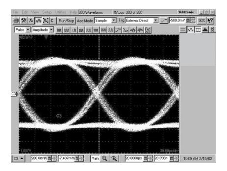
Figure 3: Oscilloscope display of an eye pattern
