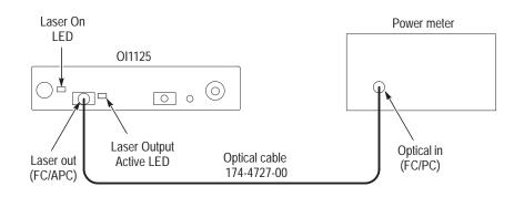
Figure 12: Setup for the output power test
